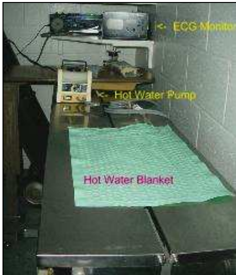
Figure 1. Hot water “Blanket”
